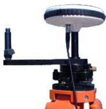
Allowing for kinematic initialization using Initializer bar at the base
